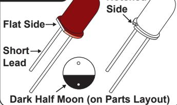
There are three main ways to determine the cathode side of the LED. The Parts Layout will indicate the cathode side of the LED by a dark half moon shape. On the physical part, usually, the cathode can be identified by one of three ways:
